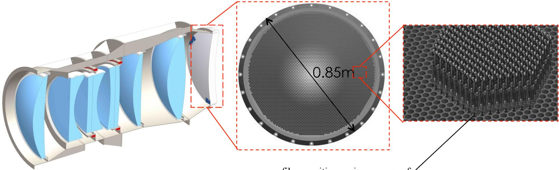
fiber positioners in an array of precision holes in the focal plate
